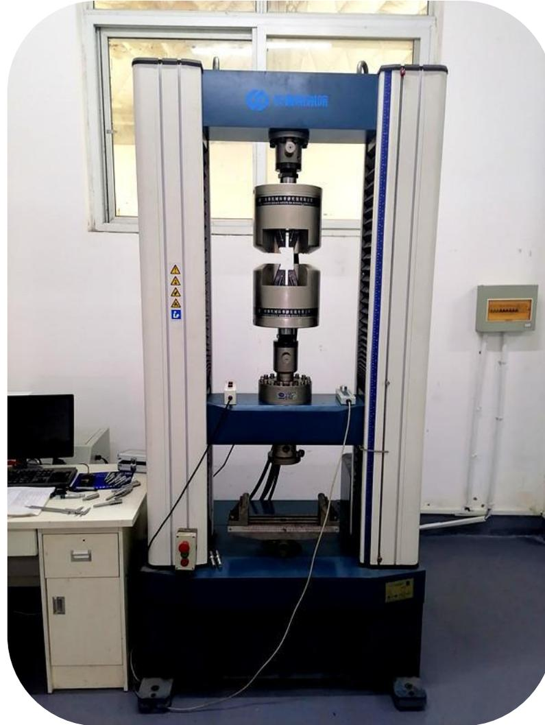
Mechanical tensile tester
