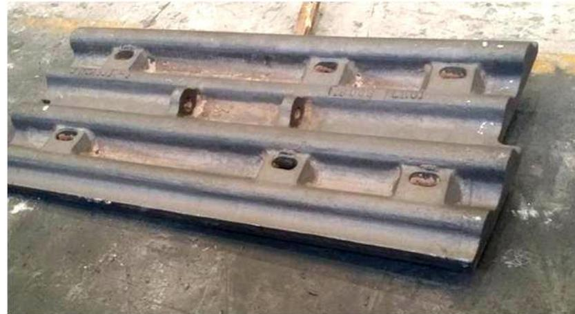
$\Phi 6.7 \times 11.58\text{m}$  Ball mill shell liner
