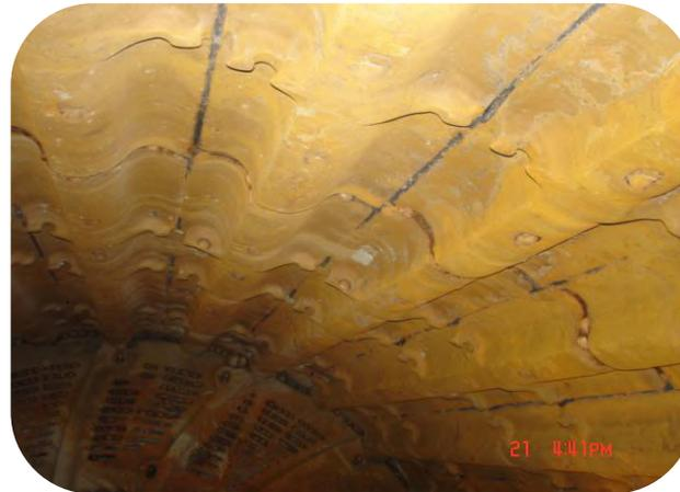
Reasonable Design: The plate of SAG gradually and evenly worn out,and the shape does not change
