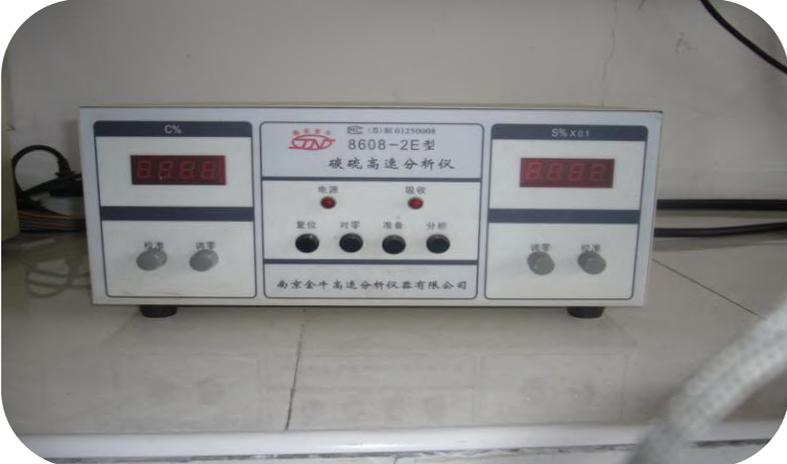
Carbon sulfur analyzer
