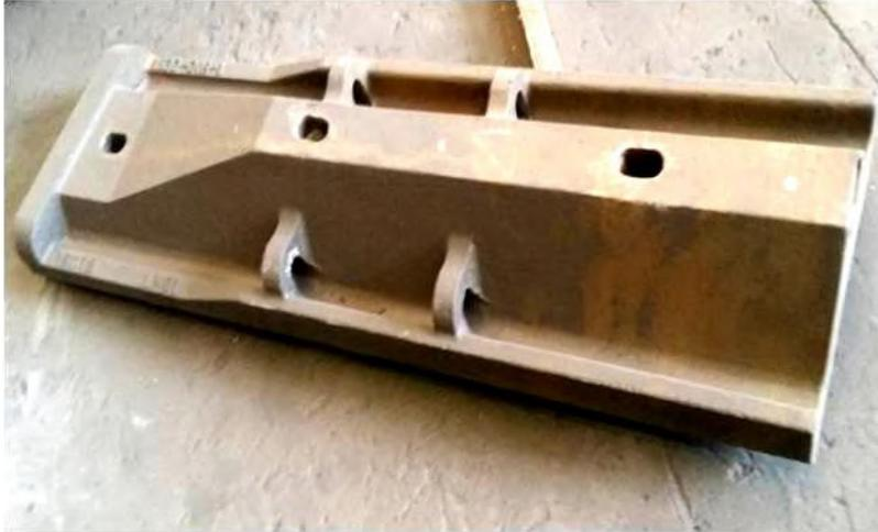
$\Phi 9.75 \times 4.57\text{m}$  SAG feed inlet liner
